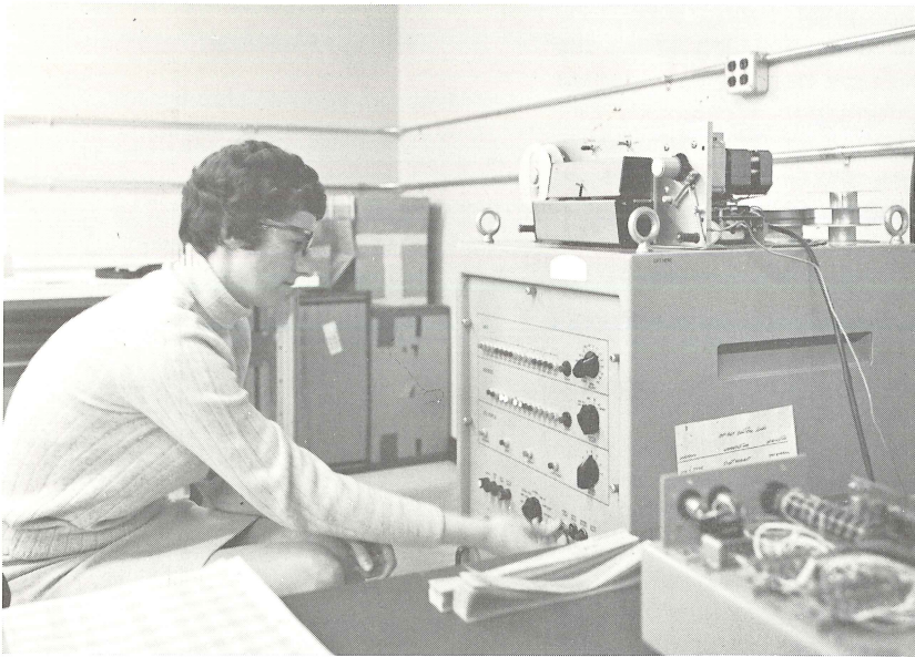
The PDP-10 tests this small computer, performing a laboratory task, while time-sharing is going on. (Right) Software for the small computer can be developed from one of the teletype terminals while the small machine is being tested.
