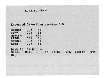
Type SYSGEN after the A> on the above screen. Then press RETURN. The system responds with the following screen:
