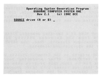
Since drive A contains the Extended Utility Diskette, press A to designate it as Source drive. Then press RETURN.
